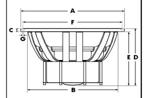
A - Overall diameter305mmB - Cut out diameter270mmC - Flange thickness6.3mmD - Overall height154.3mmE - Basket/magnet depth148mmF - Mounting holes location diameter292mm
